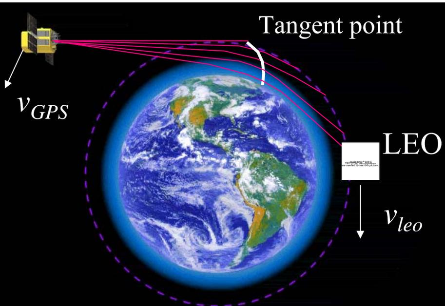
The LEO tracks the GPS phase while the signal is occulted to determine the Doppler
