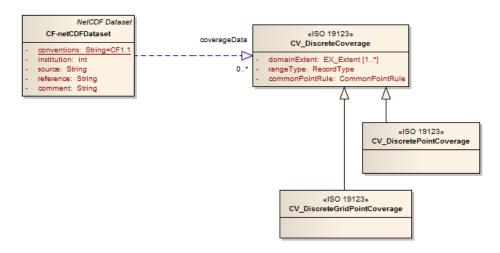
Figure 7. CF-netCDF dataset mapping to ISO coverage types
