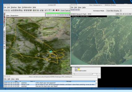
C130 flight track from Airborne Carbon in the Mountains Experiment displayed in the IDV
